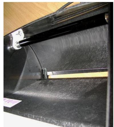
13. Once you have finished replacing the globes or the starters, replace the cover and secure it with the 4 screws. Make sure you have aligned the holes to simplify the replacing of the screws.
